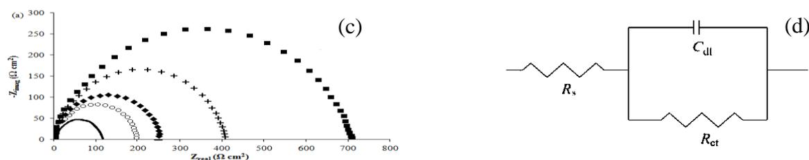
Figure 1. EIS diagrams for MS in 1.0 M HCl in the absence and presence of different concentrations of extracts of (a) *Uncaria gambir* (b) *Tinospora cripsa* and (c) *Rhizophora apiculata*. Concentrations: — 1.0 M HCl; ○○○○ 50 ppm; ●●●● 100 ppm; +++ 500 ppm and ■■■■ 1000 ppm. (d) Randle circuit diagram of corrosion mechanism.
