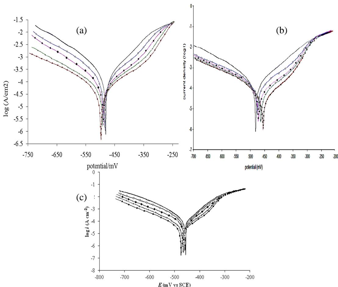
Figure 1. Polarization curves for MS in 1.0 M HCl in the absence and presence of different concentrations of extracts of (a) *Uncaria gambir* (b) *Tinospora crispa* and (c) *Rhizophora apiculata*. Concentrations: \_\_\_\_\_ 1.0 M HCl; ○○○○ 50 ppm; ●●●● 100 ppm; +++ 500 ppm and ■■■■ 1000 ppm.
