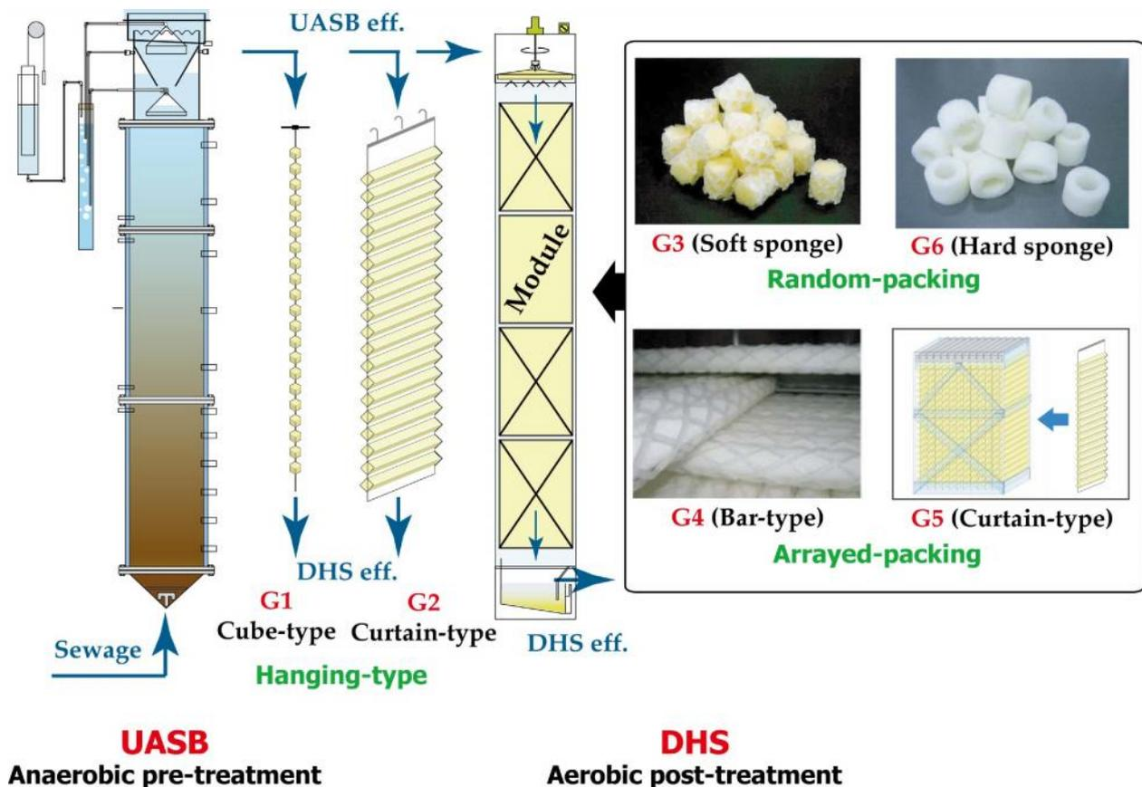
Figure 2. Configuration of DHS (generation 1 to 6)
