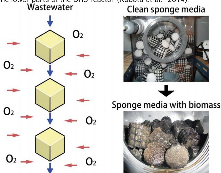
Figure 1. Concept and treatment mechanism of DHS
