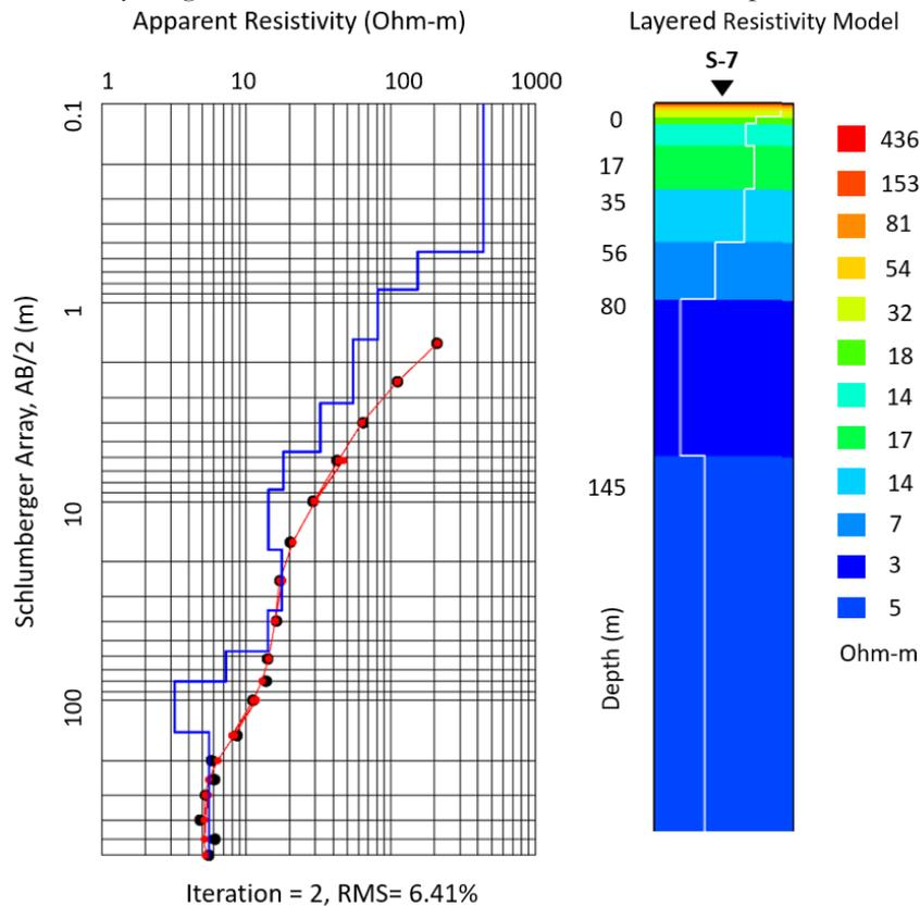
Figure 4. VES inversion model of S7 line. The contrast resistivity showed by different lithology. The RMS error of the model and data observed obtain to 6.41 % in two iteration that can be indicated as the quality of the data is really good.
