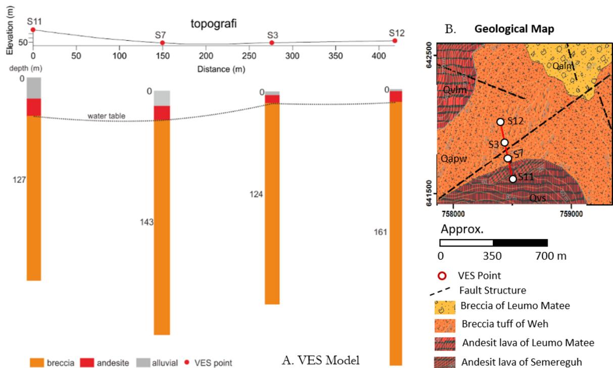
Figure 5. (A) The line section across major fault structure where groundwater is accumulated. Lithological correlation of VES model analysis (B). The line section generated topographically and correlated by the water table of the study area.
